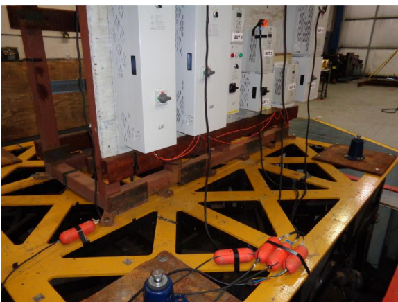
Pre-test fixture anchorage
