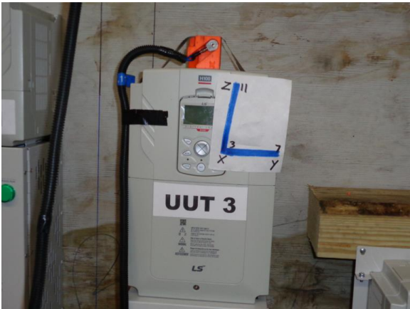
Accelerometer UUT 3 X/FB=Ch3, Y/SS=Ch7, Z/V=Ch11
