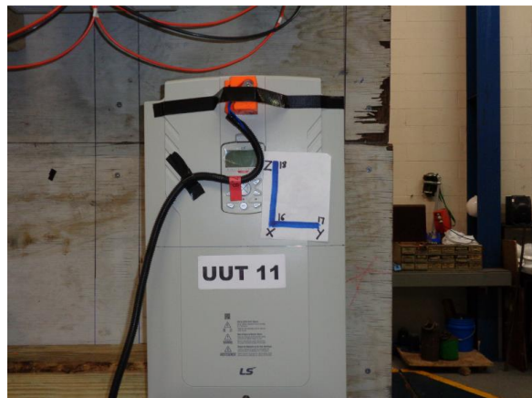
Accelerometer UUT 11 X/FB=Ch16, Y/SS=Ch17, Z/V=Ch18
