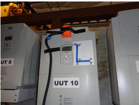
Accelerometer UUT 10 X/FB=Ch13, Y/SS=Ch14, Z/V=Ch15
